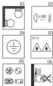
01. The fitting is suitable for fixing to the wall and to the ceiling.
