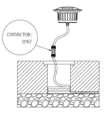
Connect the cable with the light. \*keep enough length for maintain.
