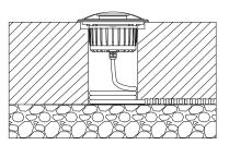
Put the light fixture into the sleeve.
